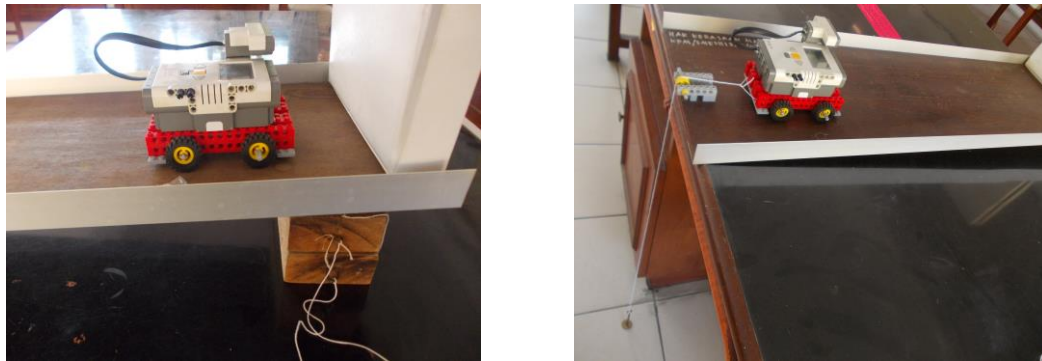
Figure 5.1 : A robot on a friction compensated runway
