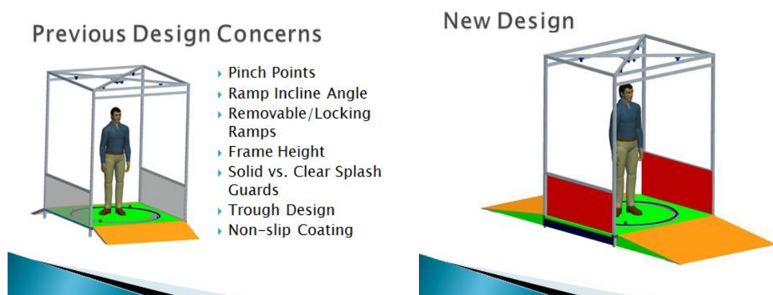
Figure 7: Some of the concerns for one of the design iterations and the final design, senior team.
