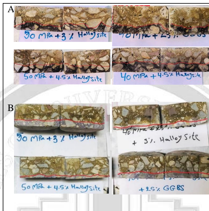
Figure 4: Chloride Migration Depth at A: 28 and B: 90 Days
