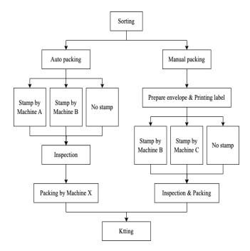
Fig. 7. Process flow of the packing line.
