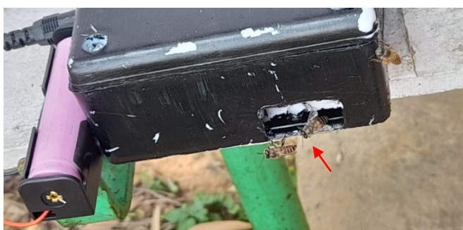
Fig 4. Bee entry and exit through the IoT device.
