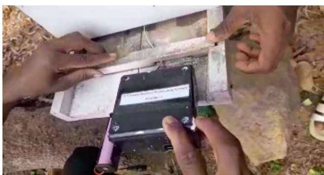
Fig 3. Integration of IoT based beehive monitoring system with beehive box.
