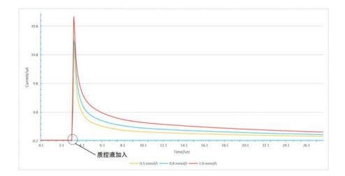
Relationship between uric acid quality control solution and response current for different uric acid concentrations at constant potential.
