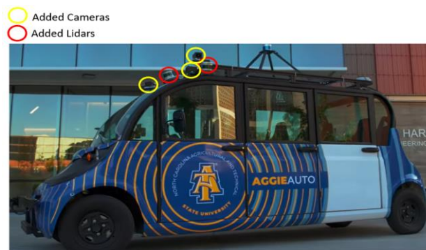
Figure 1. Added sensors to enhance the perception of the vehicles.
