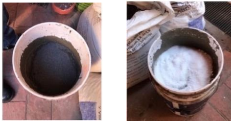
Figure 3. Concrete with fly ash (left) and nanosilica in concrete (right)
