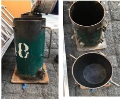
Figure 2. Molds used to make the specimens
