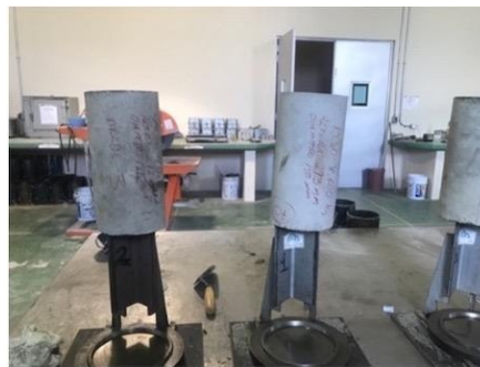
Figure 7. Arrangement of specimens prior to placement of sulfur
