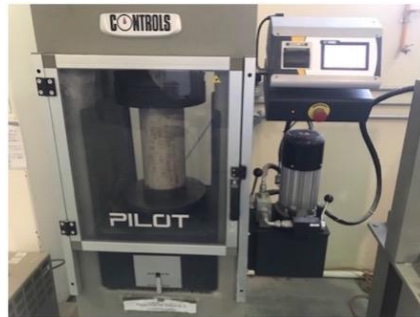
Figure 10. Compressive strength testing machine
