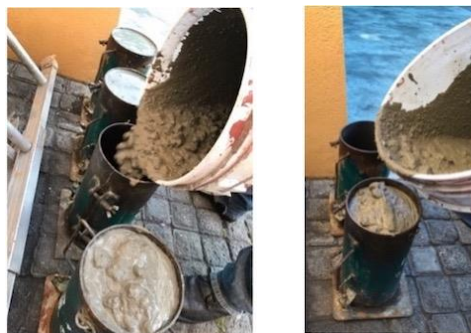
Figure 4. Pouring the concrete mixture into the molds
