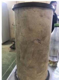
Figure 12. Fractured specimen after being subjected to the strength test
