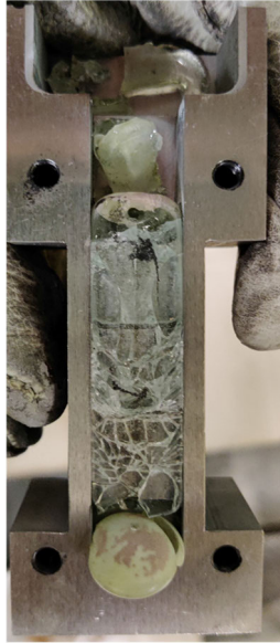
Fig. 16. Cracking observed during solidification of H2-9 flux film sample.
