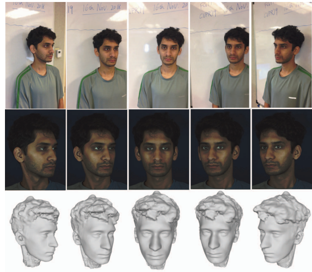
Figure 1. The montage shows selected frames of the profile to profile videos of one of the subjects, with the iPhone video on the top row, the high resolution video from the DI3D system on the middle row, and a few angles of the ground truth mesh on the bottom row.
