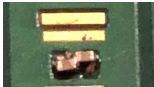
Fig. 5. 2-terminal capacitors soldered on 3-terminal pads.
