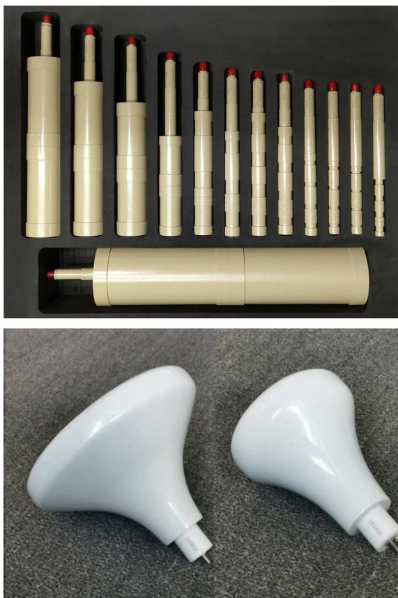
Fig. 4 dipole and loop calibration antennas.
