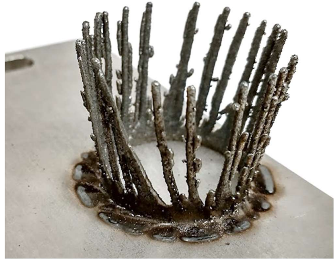
Figure 10: Open-Loop Trial of 10-Degree Cone Build
