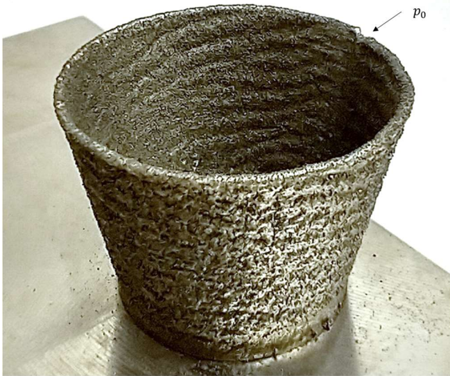
Figure 12: Closed-Loop Trial of 10-Degree Cone Build
