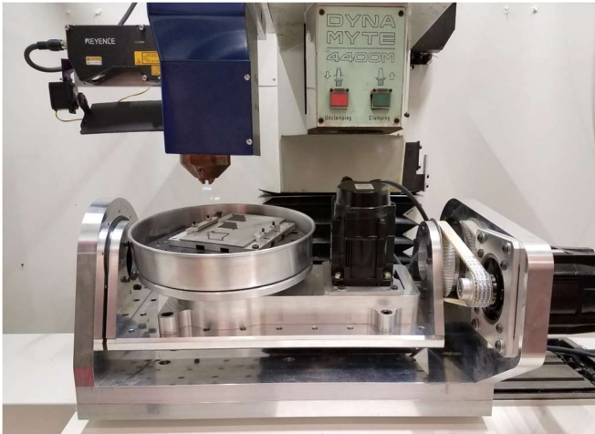
Figure 8: LENS© Five-Axis Blown Powder Machine Workspace
