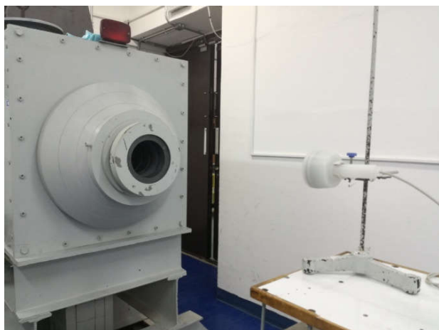
Fig. 1. The pancake G-M tube-based probe in the S-Co and S-Cs irradiation unit in the Secondary Standard Dosimetry Laboratory (SSDL) in the Vinča Institute of Nuclear Sciences.
