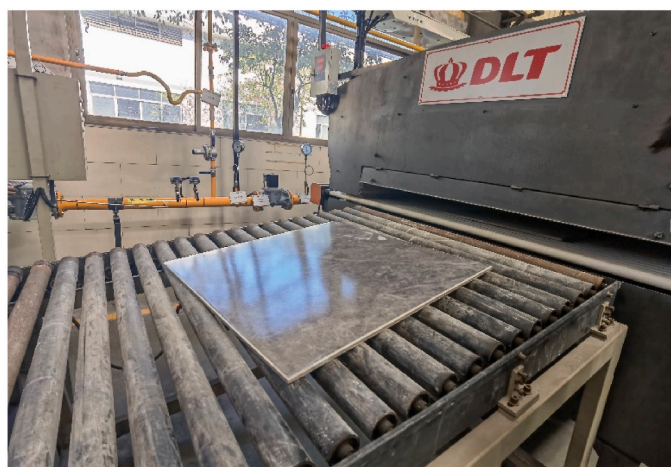
Fig. 21. Manufacturing ceramic tile with pure ammonia fuel: (a) modifications of a pilot tile production kiln for pure ammonia combustion. (b) the world's first "zero-carbon ammonia fuel made tile" rolling out of the kiln.
