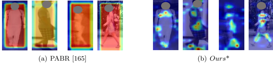
Figure 5.9: Visualization of attentive feature maps output by the pose branch of PABR [165] and the proposed method on SYSU-MM01 [194]. For each person (group), the RGB image is shown on the left and the IR image is on the right. Ours* means the proposed model is trained with identity loss and cross-modality hard triplet loss only.
