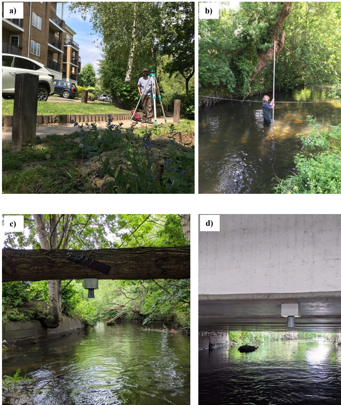
Figure 5.7: Field testing on river Wandle, London, UK. (a) Benchmark transfer using a level (b) Bathymetry survey for determining river profile and cross-sections (c) sensor installed at Wandle Main Park (upstream boundary) and (d) sensor installed at Wandle Summerstown (downstream boundary)
