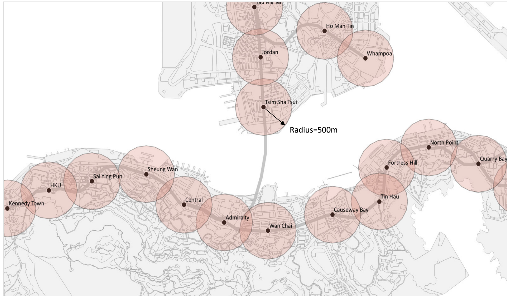
Figure 5.3: Station affected areas that are used to calculate the supplementary factors surrounding metro stations. The radius of each circle is 500 meters
