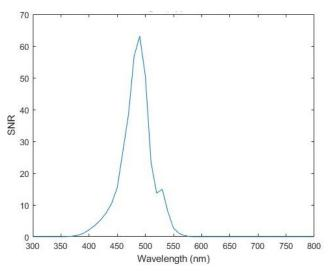
Fig 4. The SNR at 200 m distance from source in clear oceanic water.
