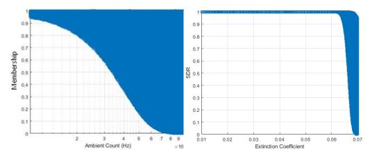
Fig 12. (left) The results of Monte-Carlo modelling between 0.03 and 0.07 extinction coefficients to produce a distribution of SDR values for ambient count rates and thus, the fuzzy set for Background Count (Bkcnt) Fig 12. (right) The converse, where ambient count rate was varied between 1Ghz and 10Ghz to understand how it effects the relationship between extinction coefficient and SDR and thus, the fuzzy set for Extinction Coefficient (ExCo).
