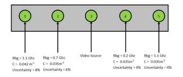
Fig 15. An abstract illustration of five nodes mounted along the pipeline, along with the parameters used for routing, before the routing has commenced.
