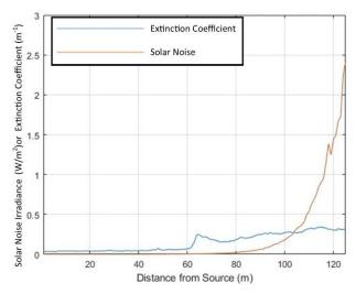
Fig 6. Solar noise and the extinction coefficient increase as distance from surface decreases.
