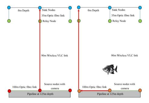
Fig 11. (left) An abstract illustration of the network route based upon the initial modelling and there is no LOS obstruction, fig 11. (right) The same except an obstruction has occurred causing the system to route around the object.
