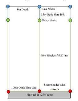
Fig 9. An abstract illustration of part of the proposed network where red circles are the source nodes, green are the relay nodes and blue are the sink nodes.
