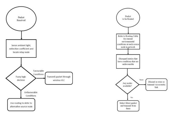
Fig 10. (left) The proposed fuzzy logic system flowchart. (right) The proposed source routing algorithm flowchart.
