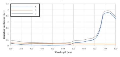
Fig 3. Extinction coefficients of type 2 wasters at visible light wavelengths where a, b and c are the absorption, scattering and extinction coefficients respectively.
