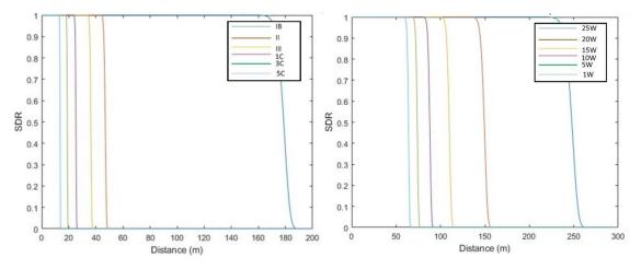
Fig 5. (left) The SDR over distance in different Jerlov Water Types, (right) The SDR over distance for different transmission powers.
