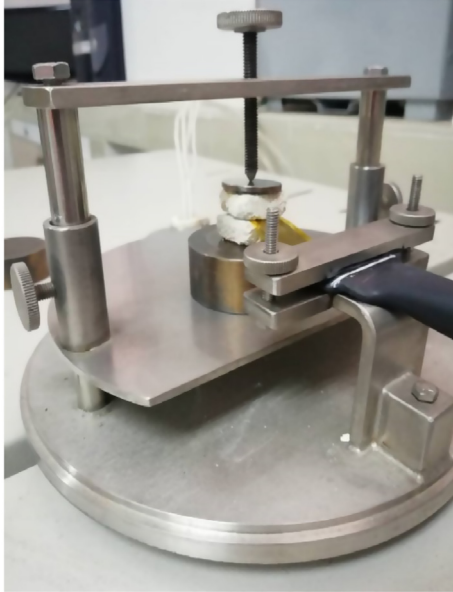
Fig. 6 – Setup for a thermal conductivity test.
