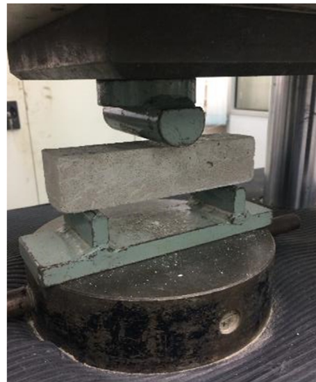
Fig. 4 – The bending test was executed on a 100 \times 100 \times 500 mm prism.
