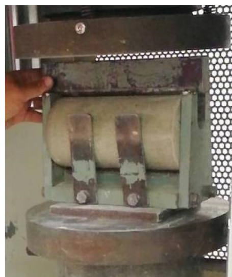
Fig. 5 – The tensile test was accomplished on a 100 mm in diameter x 200 mm in height prism.
