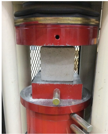
Fig. 2 – Compression test was achieved on a 100 \times 100 \times 100 mm sample.
