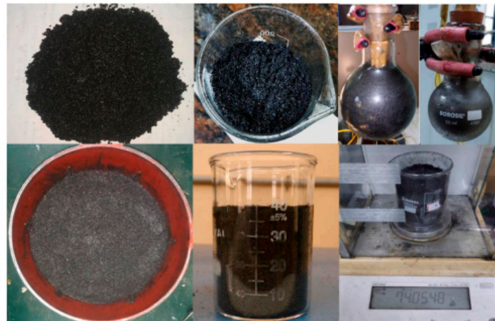
Figure 28. Macroscopic pictures of the prepared CPCM [74].
