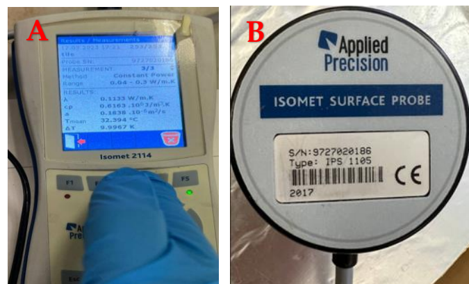
Figure 3. A) ISOMET 2114 device, and B) The surface probe of the ISOMET device.
