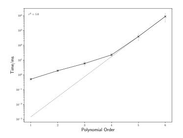
Figure 3: Run-time performance of meld as the number of terms in a tensor polynomial increases.
