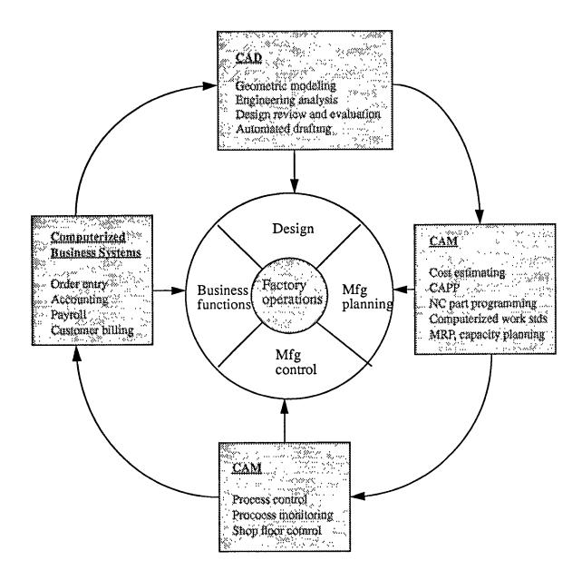
Fig 4.2 Computerized Elements of a CIM System
