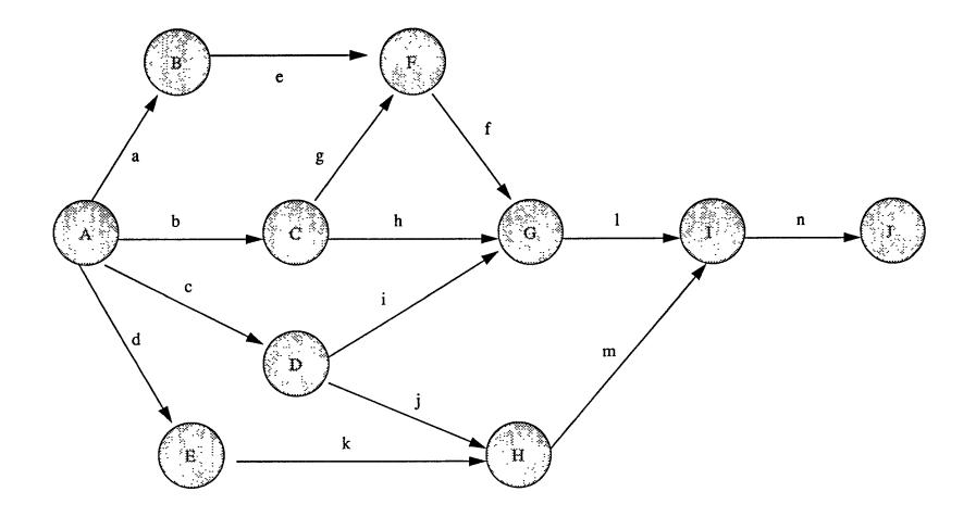
Fig. 5.8 Sequence of Operations Required to Complete a Product
