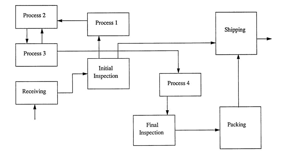
Fig 2.2 System Functions Before Integration
