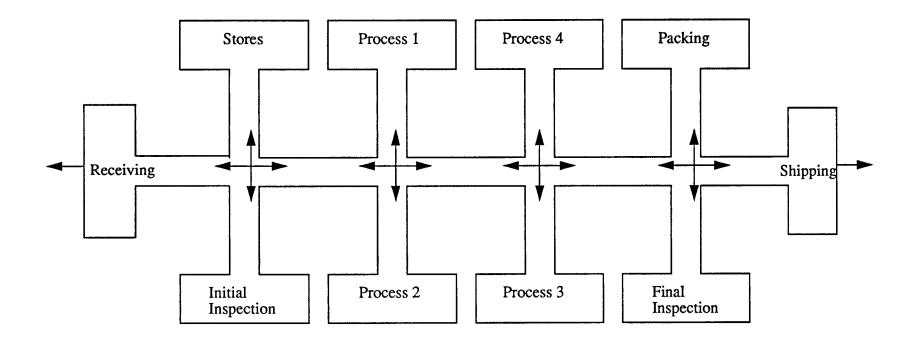
Fig 2.3 System Functions After Integration
