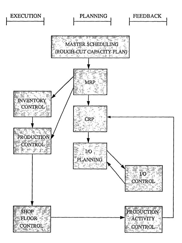
Fig. 5.2 The Manufacturing Planning and Control Process
