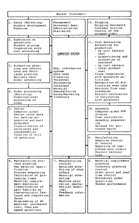
Fig 3.2 Computer Functions in Manufacturing
