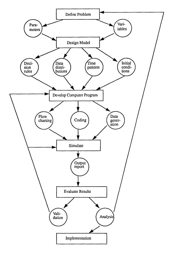
Fig 6.1 Computer Simulation Methodology
