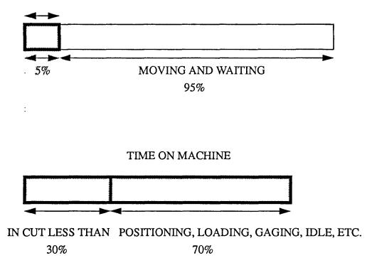
Fig 3.1 Life of the Average Workpiece in the Average Shop
