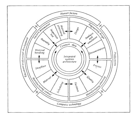
Fig 4.1 Model of a CIM System
