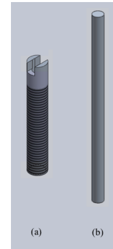
FIGURE 2. Modified Tuning Pins (MTPs): (a) Hollow M4 tuner used for a manual tuning of cavities and coupling windows; (b) Inner pin used to short circuit cavities or coupling windows by inserting it in the hollow M4 tuner.
