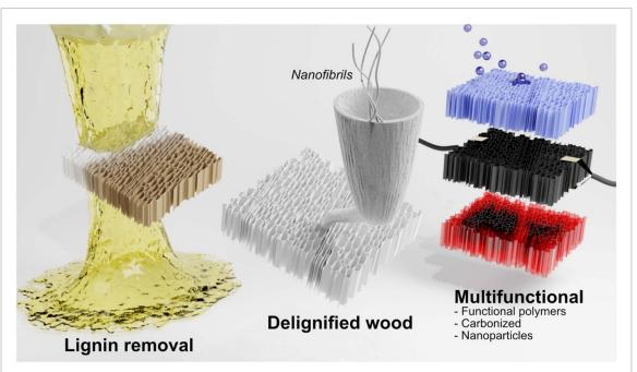
**Figure 7.** Scheme for top-down preparation of wood nanomaterials. Lignin is removed to form a nanoporous, delignified wood substrate. This can be functionalised by, for instance, polymers, nanoparticles or by carbonisation. Reproduced from [45]. CC BY 4.0.
