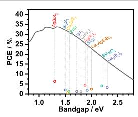
**Figure 21.** Difference between best PCE values reported for Bi-based PV devices and the corresponding Schockley–Queisser limit. PCE were obtained from [162–164] (AgBi<sub>x</sub>I<sub>y</sub>, Cs<sub>3</sub>Bi<sub>2</sub>I<sub>9</sub>, Cs<sub>2</sub>AgBiBr<sub>6</sub>) [165], (Bi<sub>2</sub>S<sub>3</sub>; Cu<sub>x</sub>BiS<sub>y</sub>; AgBiS<sub>2</sub>) [166], (BiI<sub>3</sub>) [167], (BiSI) [168], (BiOI) and [169] (BiFeO<sub>3</sub>).
