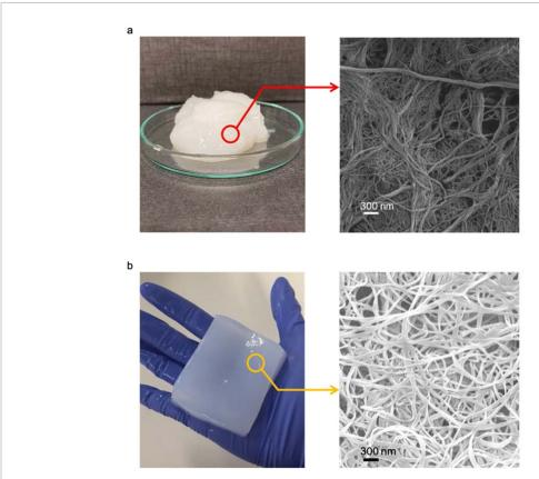
**Figure 16.** (a) An aqueous gel of nanocellulose consisting of ca. 98 wt.-% water, along with a high magnification scanning electron microscopy (SEM) image showing the morphology of the nanocellulose; (b) BC pellicle with a water content of 99 wt.-% and an SEM image showing the morphology of BC. Reprinted from [139], Copyright (2020), with permission from Elsevier. Reprinted with permission from [140]. Copyright (2019) American Chemical Society.
