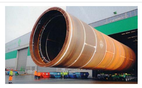
Figure 20. A 1302.5 tonne monopole. Reproduced with permission from [159]. [Source: EEW SPC].
