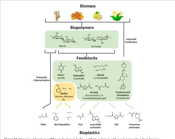
Figure 12. Overview of bioplastics (BPs) production including synthetic polymers with novel composition from biomass feedstocks.
