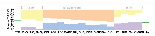
Figure 22. Band edge energies offset of several Bi-compounds along with conventional electron- (ETM) and hole-transporting materials (HTM) [165, 170]. CBI, ABS, CABB, ABI, BPS and F8 stand for  $Cs_3Bil_9$ , AgBiS2,  $Cs_2AgBiBr_6$ , Ag\_3BiI\_6, BiPS\_4 and poly(9,9-di-n-octylfluorenyl-2,7-diyl), respectively. Reprinted with permission from [170]. Copyright (2020) American Chemical Society.
