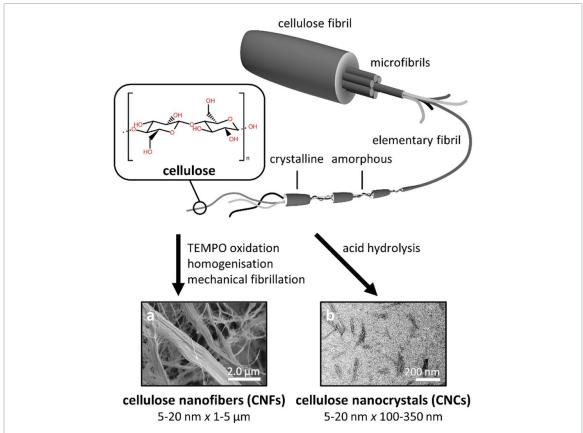
**Figure 5.** Naturally occurring cellulose fibrils comprise a hierarchical structure, allowing for nanocellulose to be extracted in the form of either (a) high aspect ratio CNFs or (b) colloidally stable CNCs. Images courtesy of Yating Zhang and Thomas Parton.
