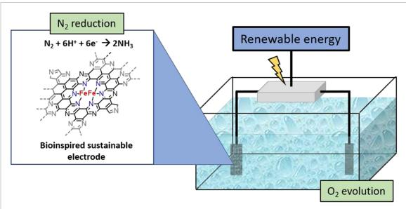
Figure 26.  $NH_3$ -producing electrolyser with a bioisnspired material acting as a working electrode where the  $N_2$  reduction takes place:  $N_2 + 6 H^+ + 6 e^- \rightarrow 2 NH_3$ .  $O_2$  evolution occurs at the anode:  $2 H_2O \rightarrow O_2 + 4 H^+ + 4e$ .
