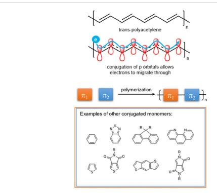
**Figure 14.** Top: Illustration of how extended  $\pi$  orbitals in CPs function. Bottom: select monomers used to construct CPs with different properties determined by the structure of the conjugated backbone.
