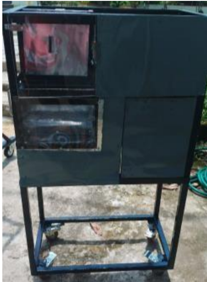
Figure 7. Final product of the developed multifunction leaves stem cutting machine
