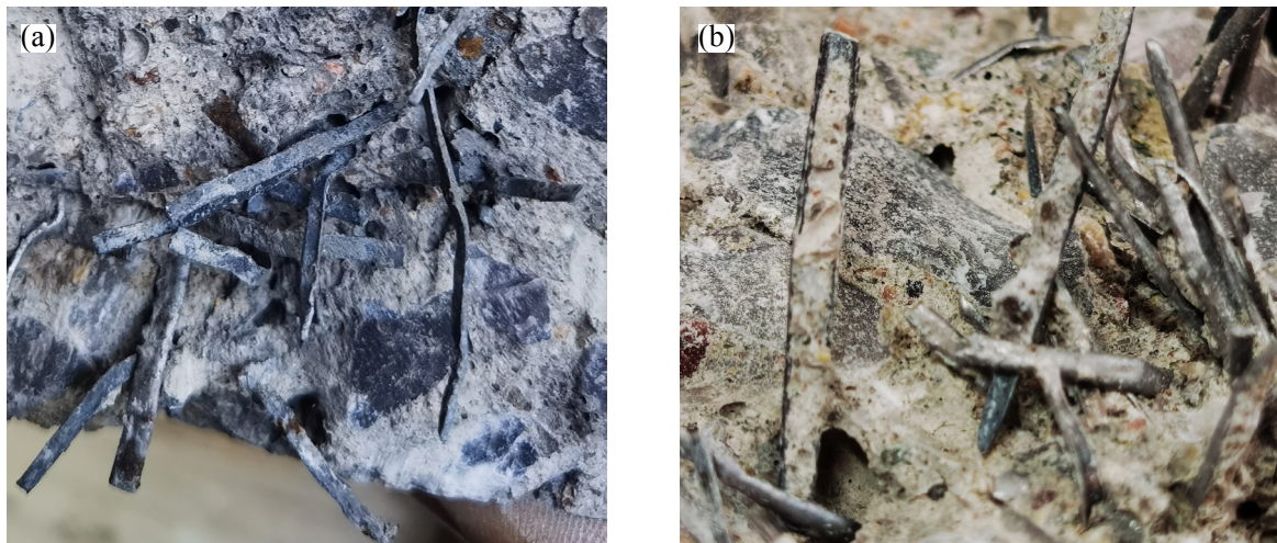
FIGURE 11. Fibers view on broken section of the bent samples: (a) F0J20; (b) F20J0.
