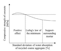
**FIGURE 9.** Hypothesis for the compressive strength of concrete as a function of standard deviation of water absorption of recycled coarse aggregate (when the mean value is constant).
