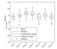
FIGURE 7. Cube compressive strength evolution of concrete mixtures.
