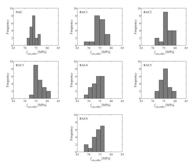
FIGURE 5. Cube compressive strength distribution of concrete mixtures.
