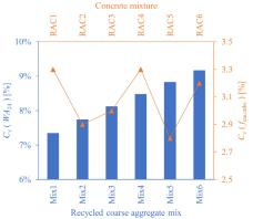
FIGURE 6. Comparison between variation coefficient of water absorption of recycled coarse aggregate mix and variation coefficient of compressive strength of concrete.
