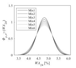
FIGURE 4. Water absorption distribution of recycled coarse aggregate mixes.
