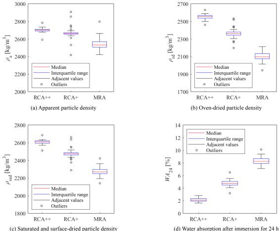
FIGURE 2. Particle density and water absorption of recycled coarse aggregates.
