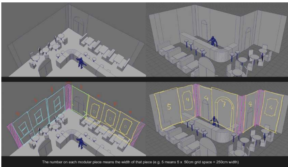
Figure 20 Example of Blockout for a Modular Environment
