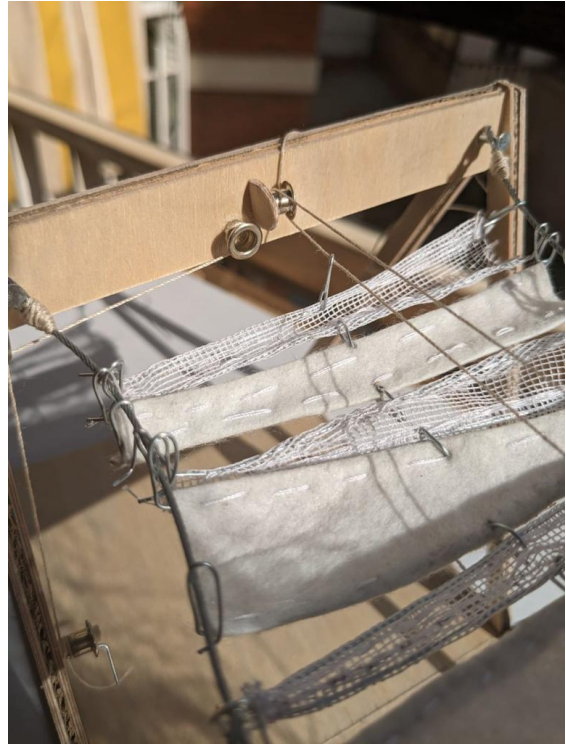
Figure 89. Detail of pulley and change of cable direction (II).
