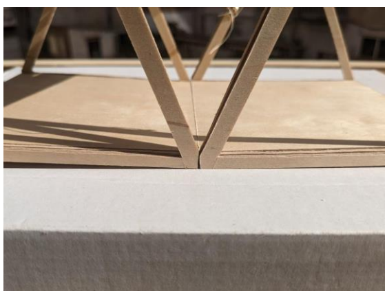
Figure 82. Wood roof fixation of the prototype.
