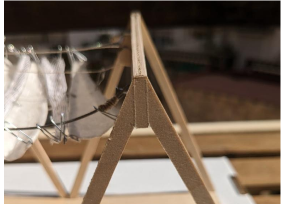
Figure 85. Joining of beam and triangular structure.
