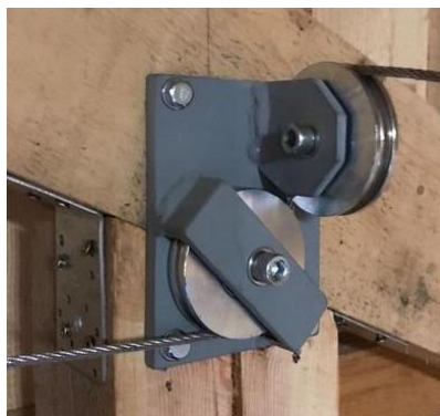
Figure 40. change of direction with rollers.
