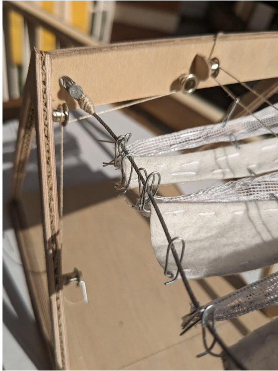
Figure 88. Detail of pulley and change of cable direction (I).
