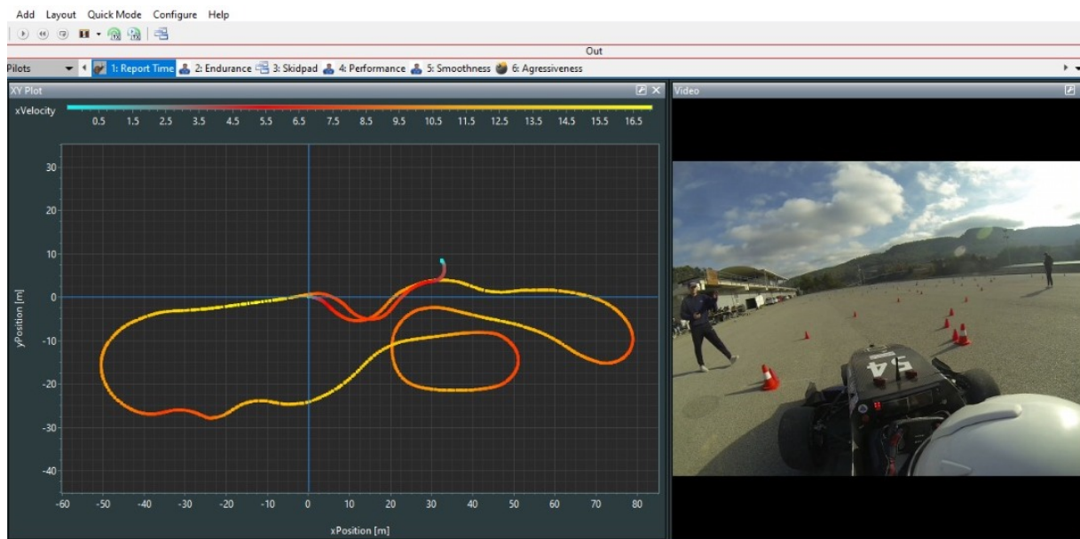
Figure 4: Dynamic visualizations with the track layout and on-board videos used last season to analyze drivers data
