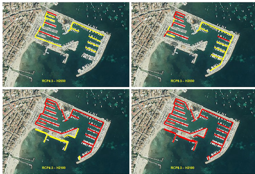
FIGURE 8 Evolution of the inoperability of berthing structures at the port of Pollença in future scenarios. Yellow: structures with insufficient freeboard; red: structures that can be flooded. Note that all the piers are inoperative in 2100 because they are fixed piers.
