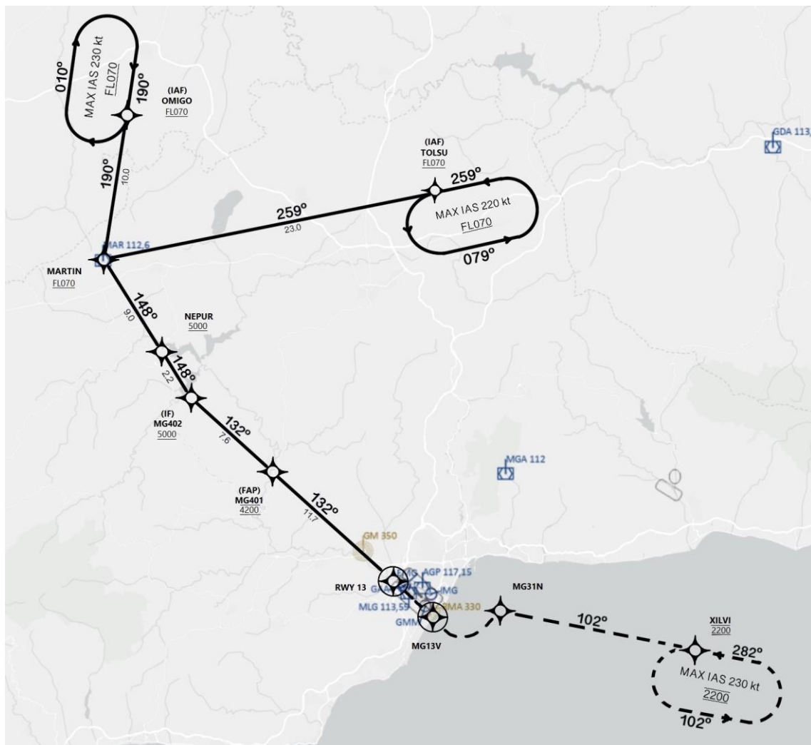
Fig. 3.23 Approach chart for the RNP APCH down to LPV minima in RWY13 of LEMG. [43]
