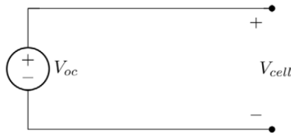
Figure 6: Ideal voltage source ECM. Adapted from [28]
