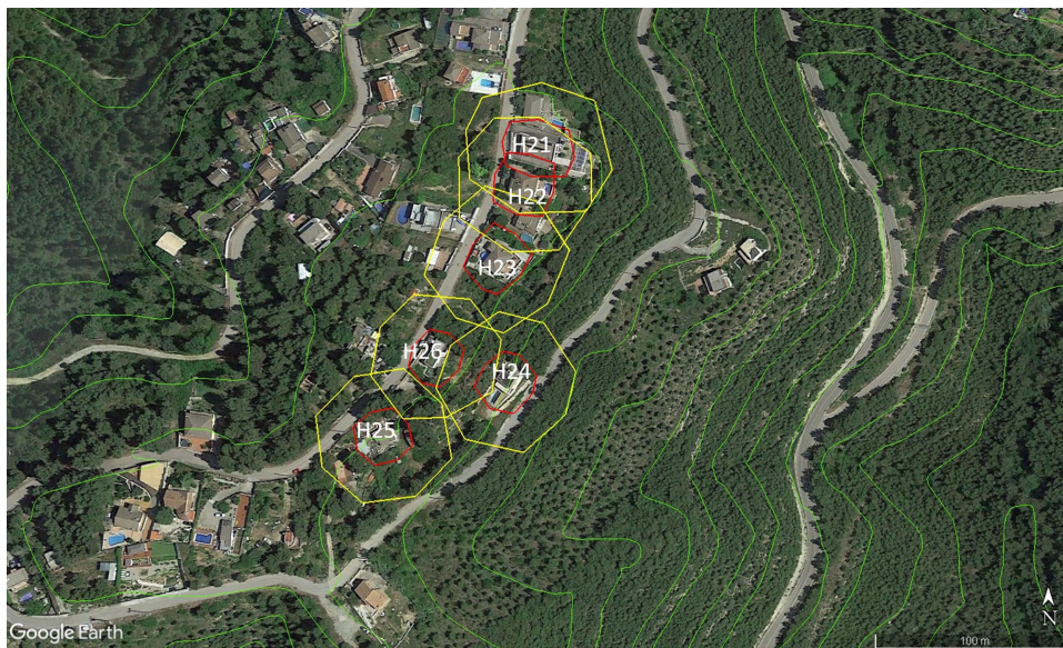
Fig. 9. Monitored properties (H21 to H26) affected by the WUI fire in El Pont de Vilomara, Spain (July 2022) (Google Earth, earth.google.com). Red line: 10 m around dwellings; yellow line: 30 m around dwellings. Green lines indicate elevation contours (Institut Cartogràfic i Geològic de Catalunya, https://www.icgc.cat/ ).
