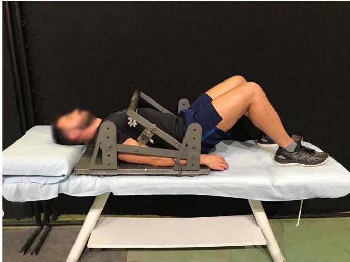
Figure 1 — The portable, one-dimensional, trunk flexor muscle strength measurement system (Measurement System). (A) The subject is assessed in a supine position with knees and hips flexed. (B) The subject is performing an isometric trunk flexion against a bar positioned on his/her chest.
