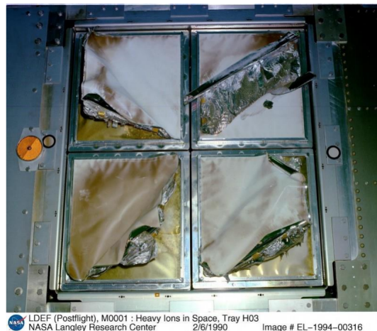
Figure 3.1: AO erosion combined with ultraviolet degradation. Extracted from NASA Langley Research Center
