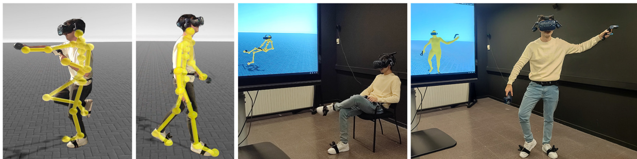
Fig. 1. Highly accurate poses reconstructed from six 6-DoF trackers. On the left, a virtual reconstructed skeleton is rendered over the user. On the right, the virtual skeleton on the screen mimics the user poses and has its end-effectors in the correct position.
