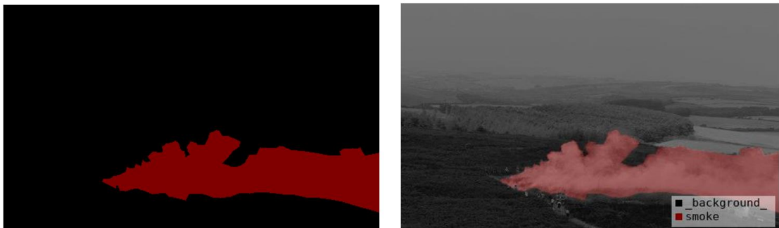
Figure 5. Image labelling example. Left: mask image. Right: class visualization of the annotation.
