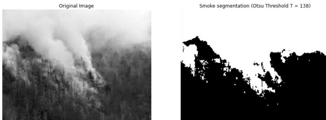
Figure 11. Smoke output for Otsu's threshold segmentation
