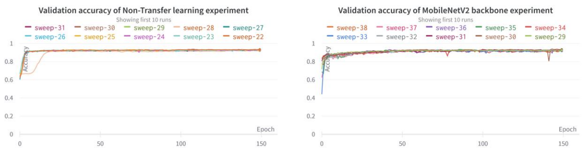
Figure 52. Validation accuracy of the 10 best parameters configurations performed on non-transfer learning tests, Left: ResNet50 backbone. Right: MobileNetV2 backbone.
