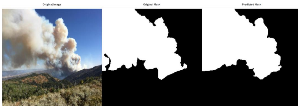
Figure 30. Smoke prediction of test_base3 (trained for 100 epochs with a LR=0.0001 and a batch size of 16)
