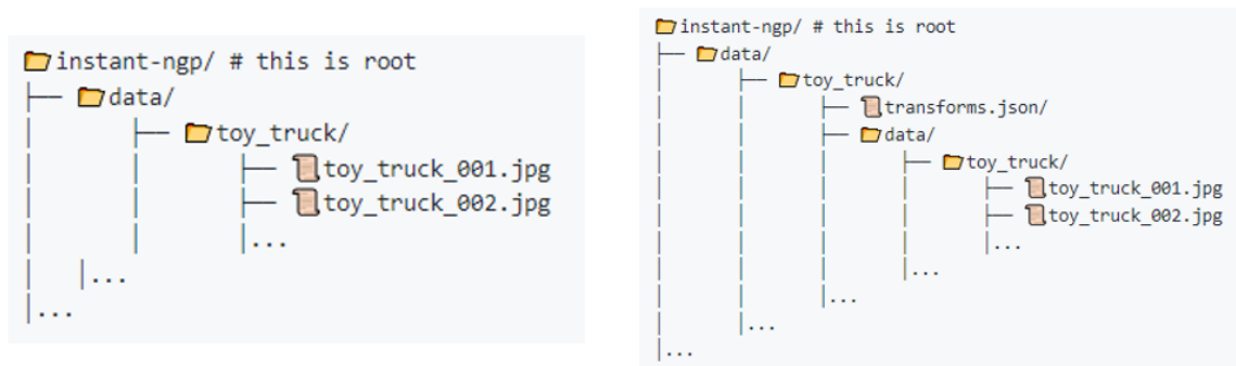
Figure 66. Data structure example for NERF 3D reconstruction. Left: file structure before generating transforms.json. Right: File structure after generating transforms.json ( Instant Neural Graphics Primitives, 2022/2023 ).
