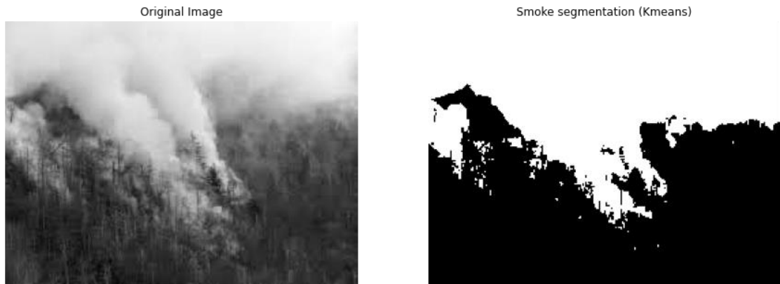
Figure 12. Smoke segmentation output for K-means segmentation
