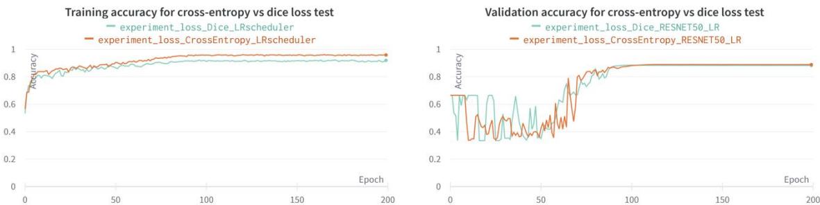
Figure 25. Training and validation accuracy performance of the loss test comparing the binary cross entropy and dice loss functions, with learning rate scheduler, tested during 200 epochs and a batch size 16.
