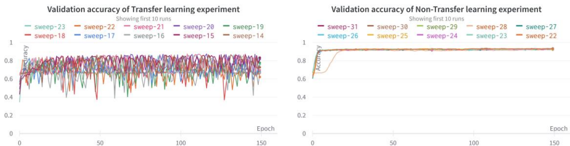
Figure 47. Validation accuracy of the 10 best parameters configurations performed on transfer learning tests, using a ResNet50 encoder. Left: with transfer learning. Right: without transfer learning.
