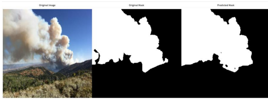
Figure 34. Smoke predictions with data augmentation of test_aug1 (trained for 100 epochs with a LR=0.0001, applying 1 augmentation)
