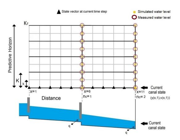
**Figure 6.** Sketch of a numerical grid of a canal with two pools controlled by two checkpoints downstream each pool. Also, it shows the x/t-dots where the flow behaviour is defined. Notice that "K" with capital letter denotes time interval of control and "k" with small letter denotes time instant of simulation.
