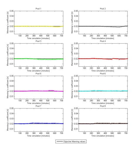
**Figure 16.** Manning's roughness coefficient trajectories obtained by FC algorithm in test 2-1 for the Corning canal (every color in the graph represent the Manning roughness coefficient calculated at every pool).
