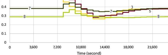
**Figure 15.** Sluicegate trajectories obtained by GoRoSoBo simplified in test 2-1 for the Corning canal (gates 3–5–7–8).
