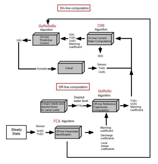
Figure 2. Overall control diagram of irrigation canal.
