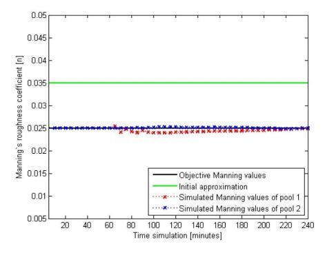
Figure 10. Manning's roughness coefficient trajectories at pools one (red line) and two (blue line) in scenario one.
