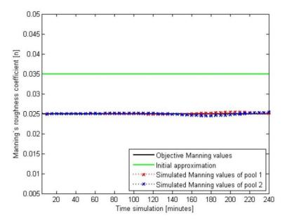
Figure 12. Manning's roughness coefficient trajectories at pools one (red line) and two (blue line) in scenario two.
