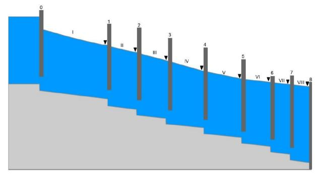
**Figure 13.** Corning canal profile. The red lines mark the position of checkpoints. The first pool is number I (so every pool in the canal has been enumerated (I–VIII)), the first checkpoint is number 1 (so every checkpoint in the canal has been enumerated (1–8)) and the triangles represent the target water level.
