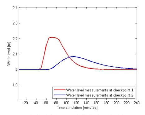
Figure 9. Water level at the checkpoints one (red line) and two (blue line) in scenario one.
