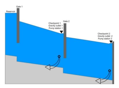
**Figure 8.** Canal profile of a canal with two pools (the arrows represent the outlet flow for the offtake orifice).
