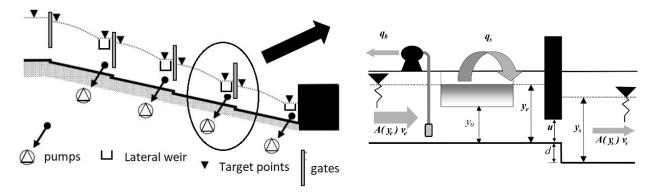
Figure 4. Example of a canal profile and diagram of a checkpoint with gate, lateral weir, and pump.
