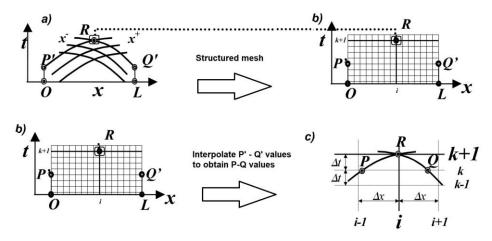
**Figure 3.** The steps for the interpolation onto a structured grid: (**a**) overlapping of the family of characteristic curves, (**b**) introducing the variables for every point (for instance P' and Q') to a structured mesh, (**c**) variables are interpolated at a particular mesh points P and Q.
