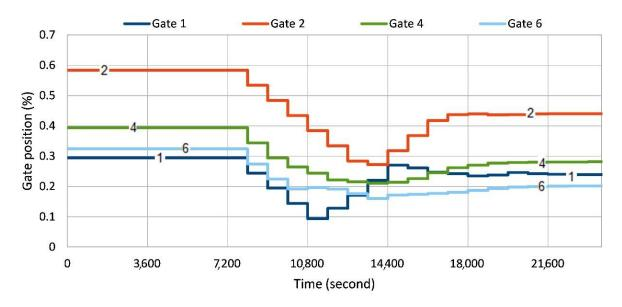
**Figure 14.** Sluice-gate trajectories obtained by GoRoSoBo Simplified in Test 2-1 for the Corning canal (Gates 1-2-4-6).
