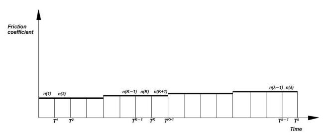
Figure 7. Mathematical representation of a Manning roughness coefficient trajectory.
