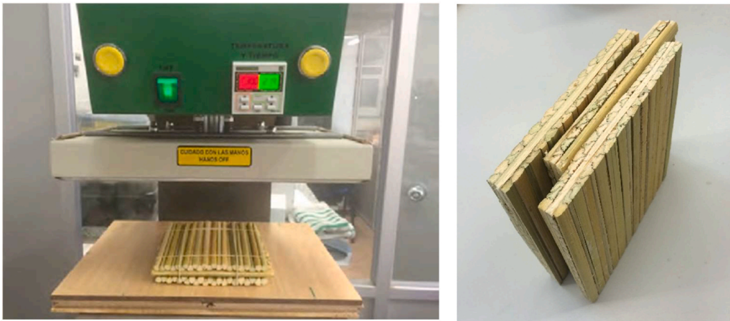
Fig. 5. Process of pressing the whole reeds.
