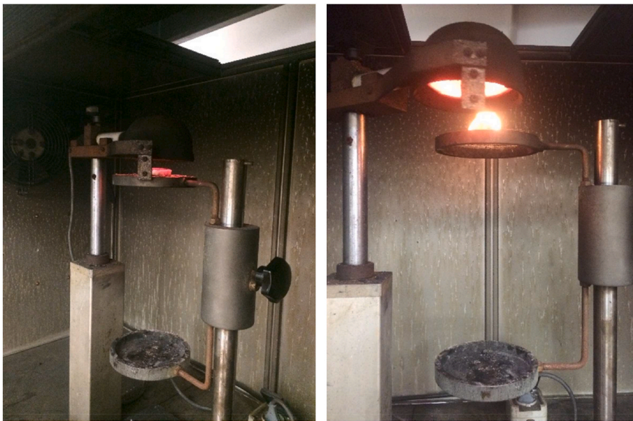
Fig. 8. A specimen being subjected to the radiator test.
