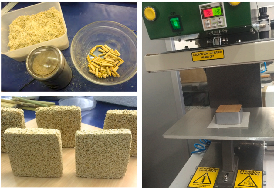
Fig. 3. Process of crushing and compacting the fibers.
