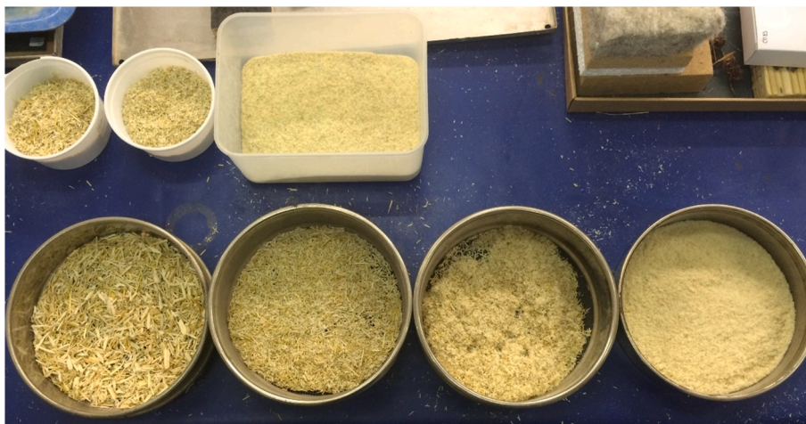
Fig. 2. Sizes and sieves of shredded fibers.
