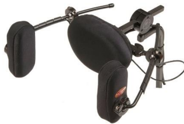
Figure 5. Head array control [17]
