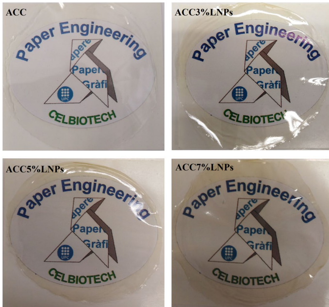
Fig. 7 Appearance and qualitative transparency of ACNC nanocomposite films with different contents in lignin nanoparticles
