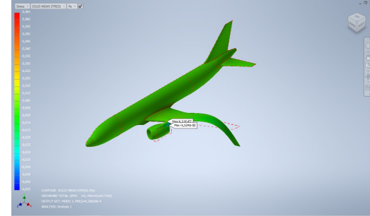
(c) Third normal mode. f = 6.588 \cdot 10^{-4} Hz
