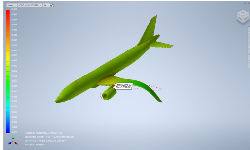
(b) Second normal mode. f = 5.276 \cdot 10^{-4} Hz
