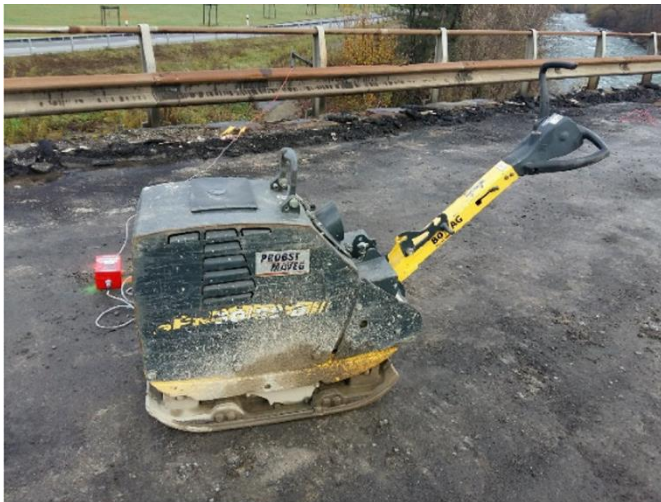
Figure 3 A portable plate vibrator has been used to generate two different levels of forced vibrations: low-frequency excitation that produce low amplitudes of vibration and high-frequency excitation that lead to higher amplitudes of vibration.
