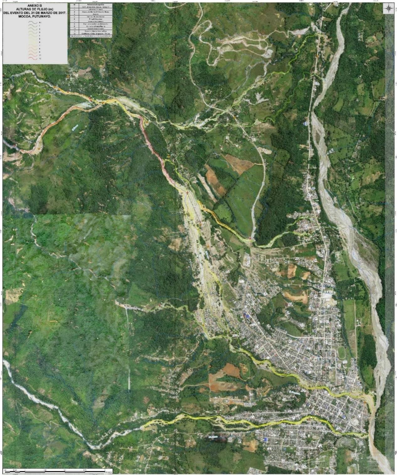
Figure 25. Flow depth map of 2017 debris flow event in Mocoa (Medina, et al., 2017).
