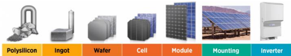
Figure 6. Stages of PV panels processing. (Source: Dawtec.com).
