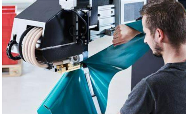
Figure 16. Welding in the production of fabric. Source: https://www.leister.com/en/Solutions/Technical-Textiles
