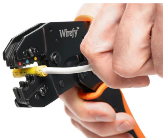
Figure 14. Example of crimping. Source: https://www.homesimprovements.net/2021/03/10/best-crimping-tool-get-it-from-wirefyshop/
