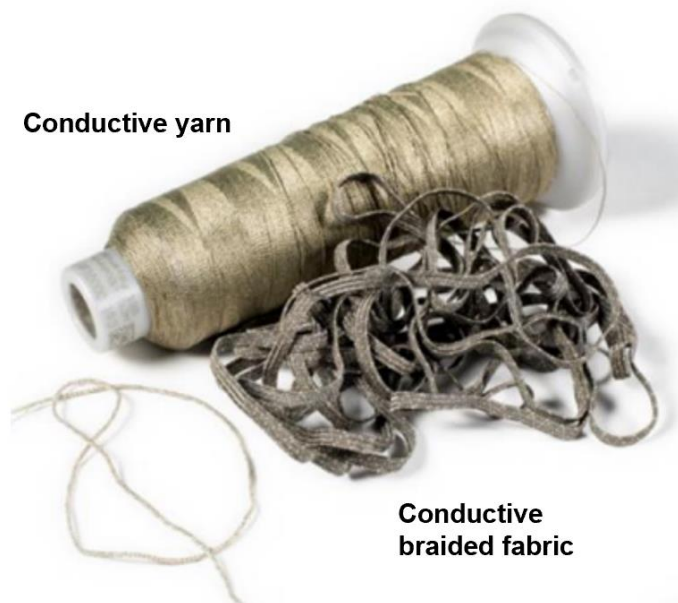
Figure 24. Examples of conductive yarns for solar textile. Source: [2]
