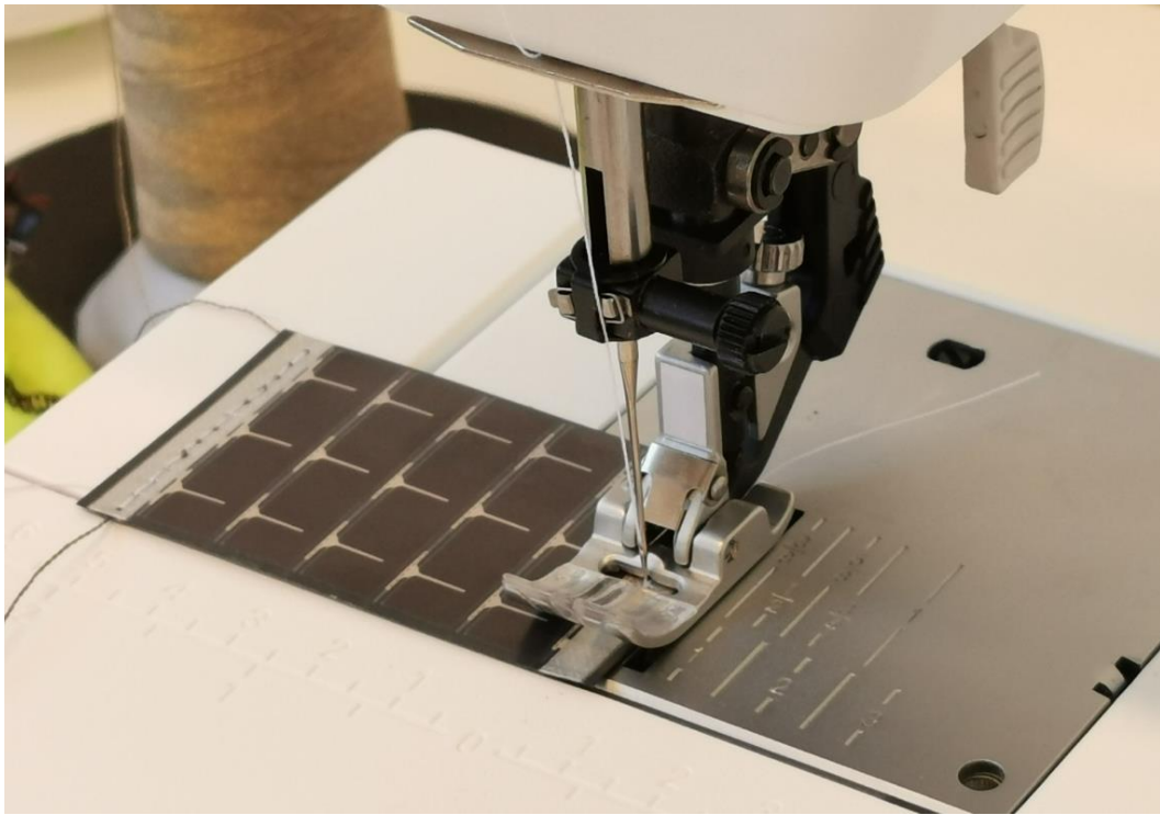
Figure 31. Stitching sewing for flexible solar cells.
