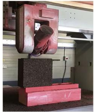
BLOCKS ARE CNC MACHINED PRECISELY TO ALLOW FOR FRICTION-FIT DRY CONSTRUCTION WITHOUT MORTAR OR GLUE
