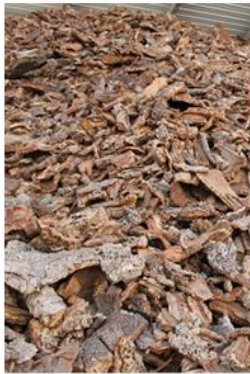
EXPANDED CORK IS MADE WITH WASTE AND BY-PRODUCT FROM CORK FORESTRY AND CORK INDUSTRY
